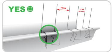
ECOCLIPS 3 is fixed by simply clipping on the outer profile of the gutter.
